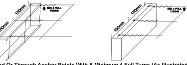
All Longitudinal Wires To Be Passed Around Or Through Anchor Points With A Minimum 4 Full Turns (As Illustrated Above) Fastening of mesh laps should be carried out from underneath
